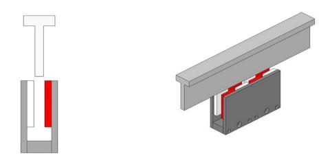
Figure 1: Brake is Completely Disengaged.
